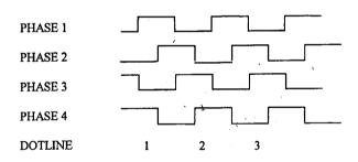
There are four different positions for the stepper motor. The driving is bipolar and can be achieved with circuits like Rohm BA6845FS. Please refer to the IC's data sheet for further informations. It is recommanded not to exceed 0.2v like voltage drop in the stepper motor driver circuit.
